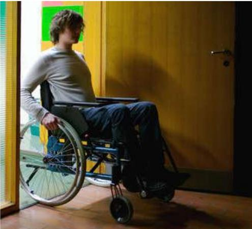
In order to accommodate a standard width wheelchair, doorways should be a minimum of 32" wide. If the doorway is located in the typical hallway and requires turning a wheelchair, you'll need a 36" door. It can be difficult to open a swinging door without a clear floor space (18-24") on the pull side of the door. An alternative could be the installation of an automatic door opener, but they are more expensive.
